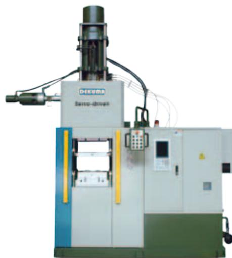
DEKUMA RVSe Series Servo-driven Energy Saving Rubber Injection Machine
